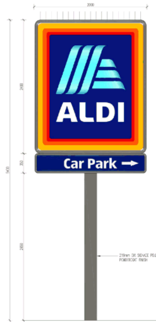
SIGN 1A, 1B DESCRIPTION: POLE MOUNTED INTERNALLY ILLUMINATED LED SIGN 2400 (W) x 2400 (H) x 60mm (D) DOUBLE SIDED "CAR PARK" SIGN: 2400 (W) x 200mm (H) DOUBLE SIDED
