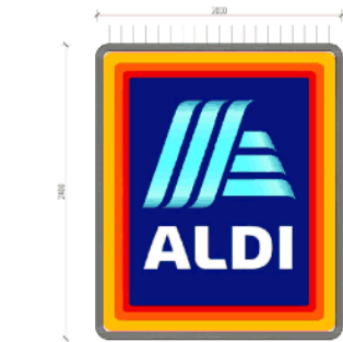
SIGN 2A, 2B, 2C, 2D, 2I DESCRIPTION: WALL MOUNTED INTERNALLY ILLUMINATED LED SIGN 2400 (W) x 2400 (H) x 70mm (D) DOUBLE SIDED
