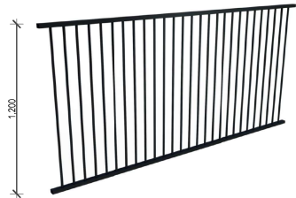
FENCE TYPE 4 - FM4 DESCRIPTION: OPEN METAL FENCE BLACK POWDERCOAT FINISH LOCATION: FRONT BOUNDARY & BETWEEN PLAYGROUNDS
