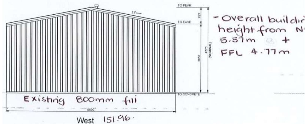
Figure 7 - Proposed west elevation
