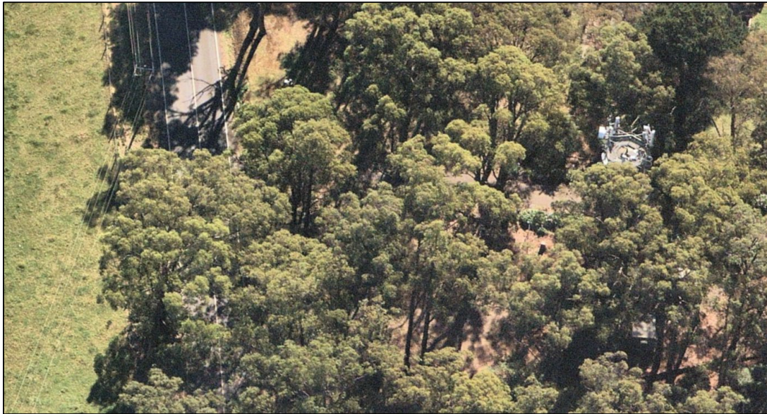
Figure 9: A 40m tower is required at this location in order to clear surrounding vegetation and terrain obstacles. The trees in the vicinity of the proposed facility are significant (refer Figures 6-8); additionally, trees near the existing facility are known to be impacting its service at a height of 25m (Nearmap)
