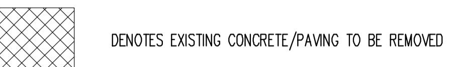
DENOTES EXISTING CONCRETE/PAVING TO BE REMOVED
