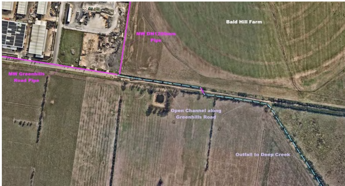
Figure 5: Current Melbourne Water constructed drains and open channels – Greenhills Road to Deep Creek. (Aerial image: Nearmap)
