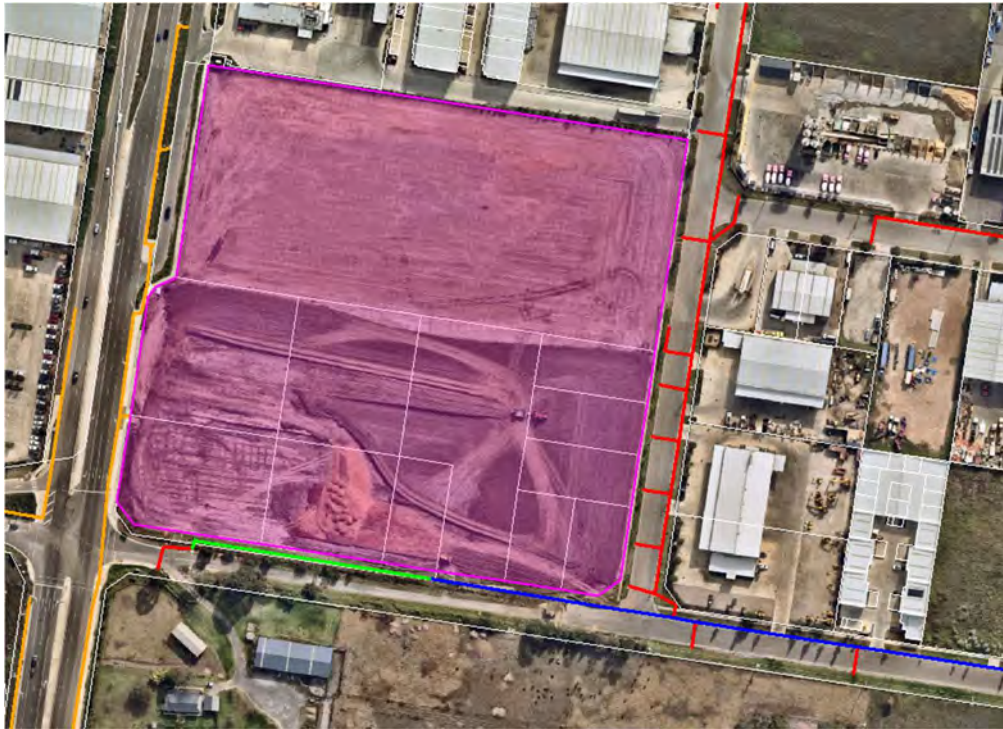
Figure 8: Existing and proposed drainage network. Existing Council pipes (red), Existing MW pipes (blue) and Proposed augmentation (green) (Source: Nearmap)
