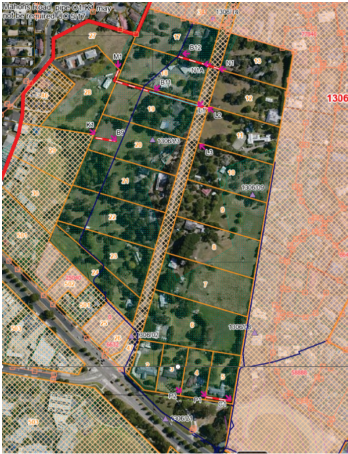
Figure 42 - Plan showing the existing Melbourne Water underground scheme drains in dark blue and proposed drainage pipes blue and dashed red lines. Source: Melbourne Water Predevelopment Advice.
