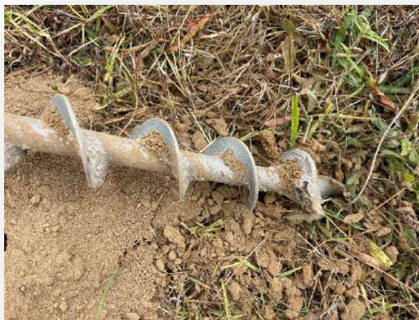
On-site Orange Brown Chromosols at 126 Bourkes Creek Road, Pakenham Upper
