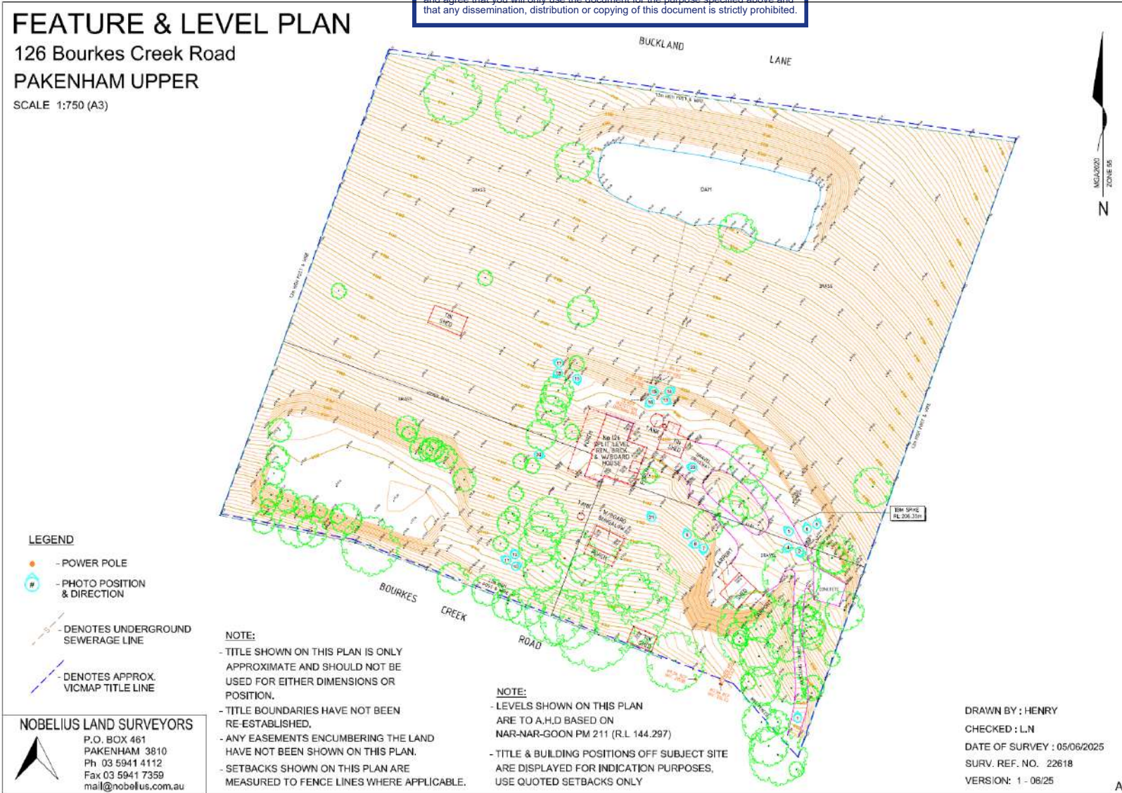
Figure 2 Feature and Level Plan showing existing conditions
