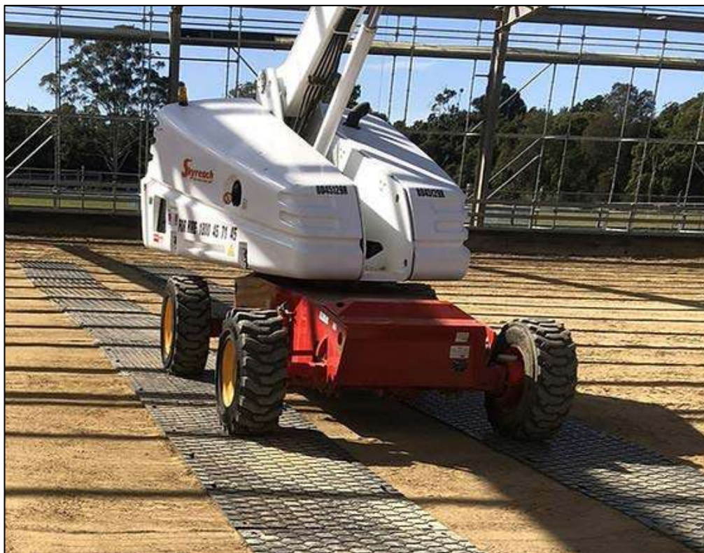
Figure 4 - Scissor lift using truck/bog mats which can protect the ground.
