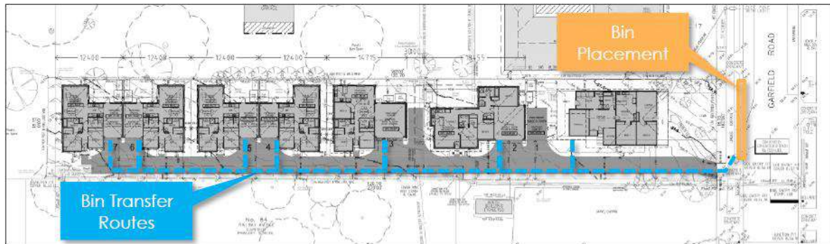
Figure 12 – Insert from enclosed Waste Management Plan noting the sites bin storage locations and collection details (Onemilegrid).
