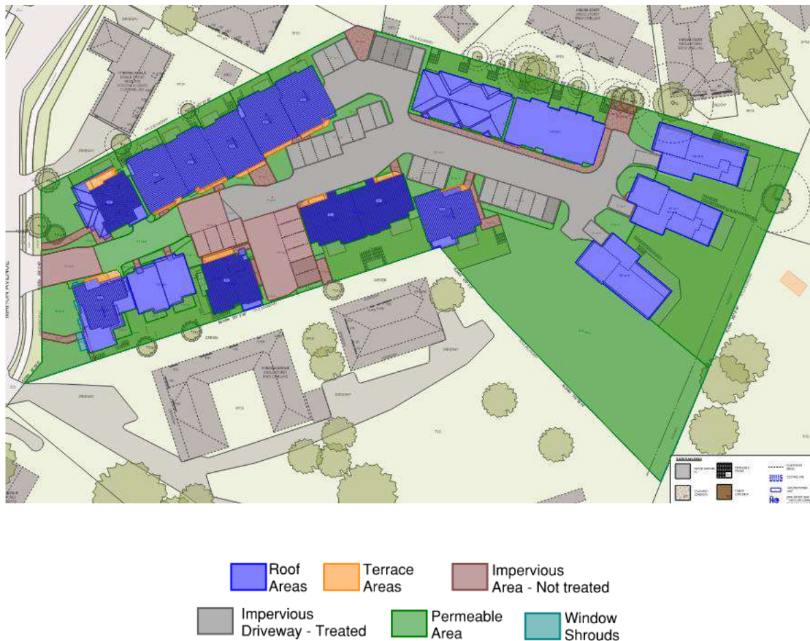
Figure 1 - Mark-up of water catchment and impervious areas
