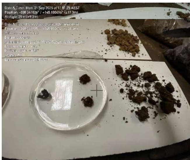
Figure 9.3 Partial Emerson Class Evaluation at Finish after 10 minutes suggests slaking and No dispersion.
