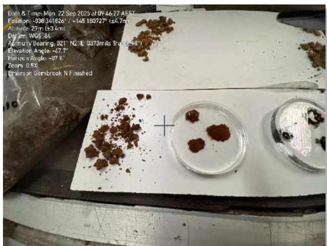
Figure 9.2 Partial Emerson Class Evaluation at Finish after 10 minutes suggests slaking and No dispersion.
