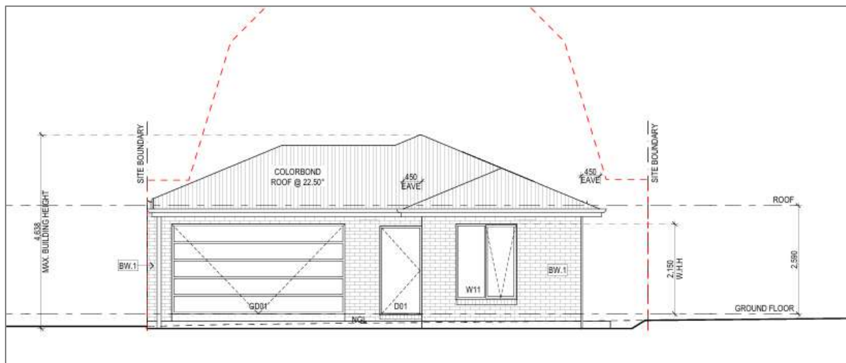
Figure 3: Front Elevation of Proposed Dwelling
