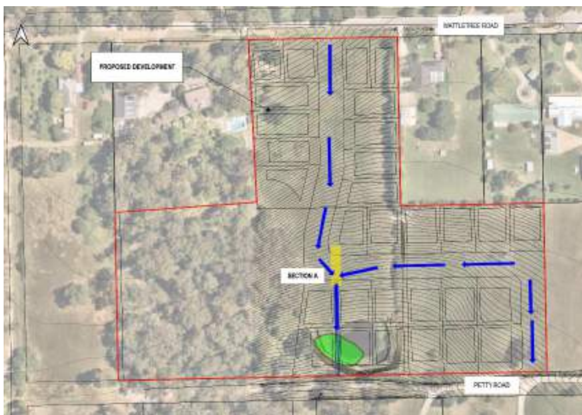
Figure 16 – Overland flow path of the proposed development
