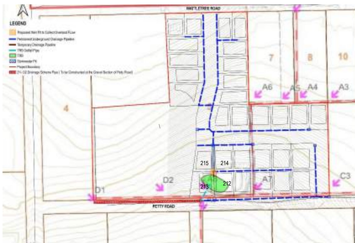
Figure 12 – Drainage alignment in the interim condition showing the concept design of the temporary retarding basin
