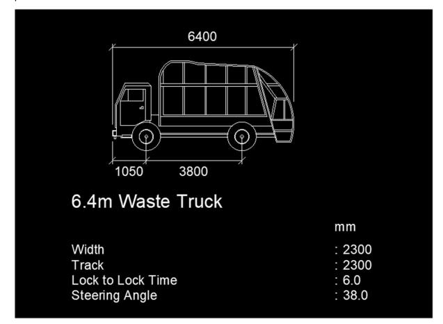
FIGURE 5: 6.4M REAR LOADER TRUCK SPECIFICATIONS (SOURCE: WASTE WISE)
