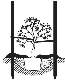
TREE PLANTING/BRACING DETAIL
