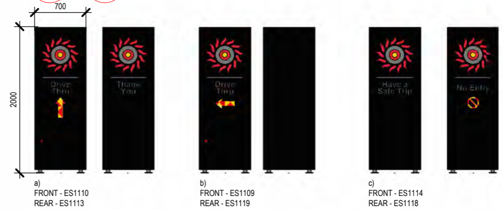
SIGN ID: ES1102 BUSINESS IDENTIFICATION SIGN INTERNALLY ILLUMINATED DIRECTIONAL AREA: 1.40m 2 (EACH SIDE)
