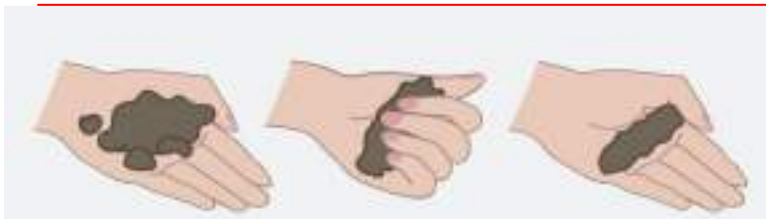
Step 1 - Prepare soil bolus and assess soil category and structure
