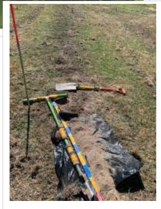
Test pit (1) showing Sandy CLAY profile
