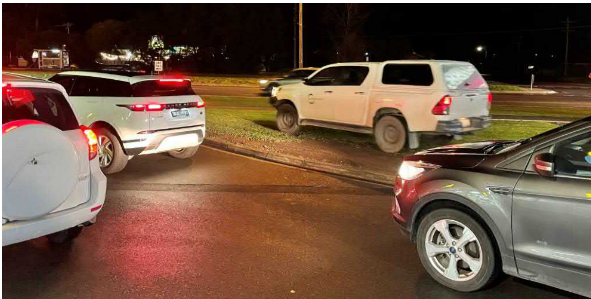
Figure 2.2: Vehicles Observed Mounting Raised Island to Bypass GYG Queue to Egress To Princes Highway
