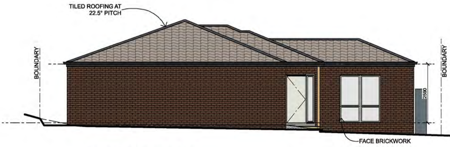
SOUTH ELEVATION 1:100 (UNIT 2)
