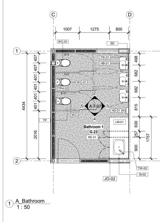
NOTE: REFER A 7.91 LINE OF HEIGHTS DRAWING FOR MOUNTING & INSTALLATION HEIGHTS AND DETAILS OF ALL FIXTURES
