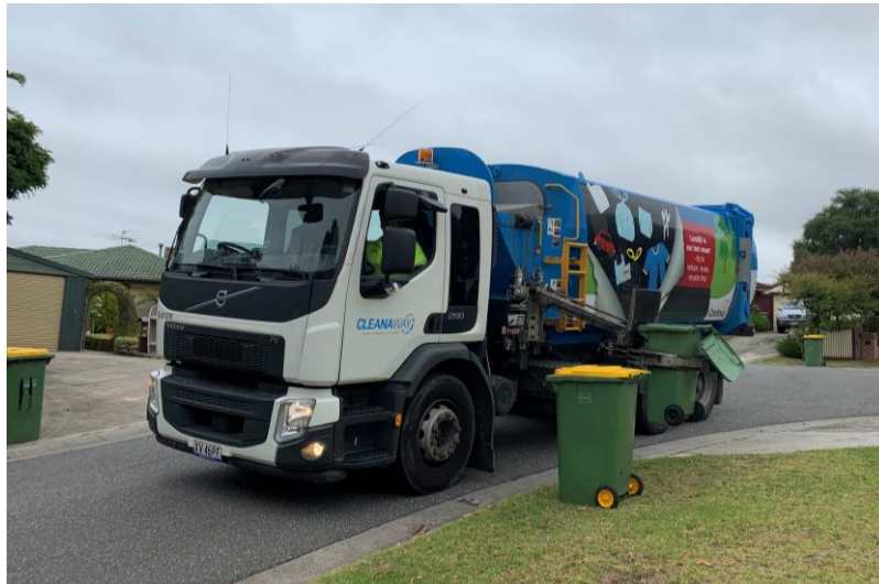
Figure 4. Example of kerbside street collections. Note: Left hand vehicle arm can extend to maximum of 3.8 metres.
