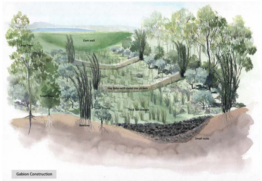
Strawbale systems for erosion control post fire
